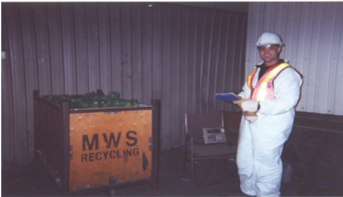
Figure 3.1 Weighing Bags of Organic Kitchen Waste at the Miller MRF in Markham
