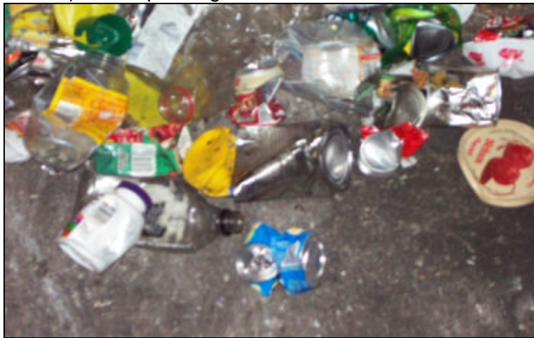
7) close-up of auger crushed container material
